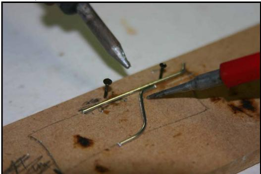
Figure 4. Soldering the corner posts.
