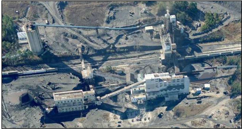
Figure 6: Oak Grove prep plant and loader; the coal from the mine arrives by an overland conveyor several miles long.
